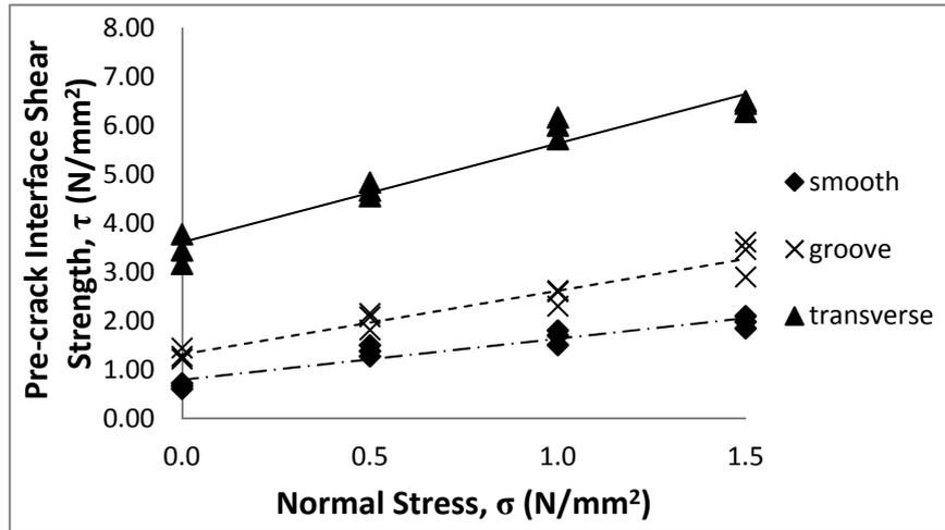
Figure 5. Relationship between interface shear strength and normal stress
