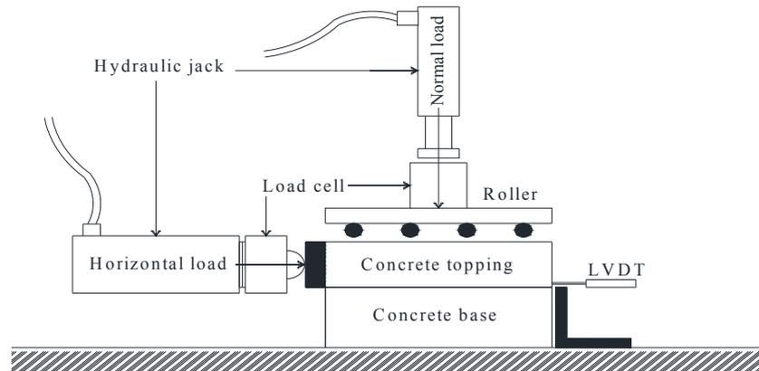
Figure 3. Schematic diagram of the "push-off" test setup
