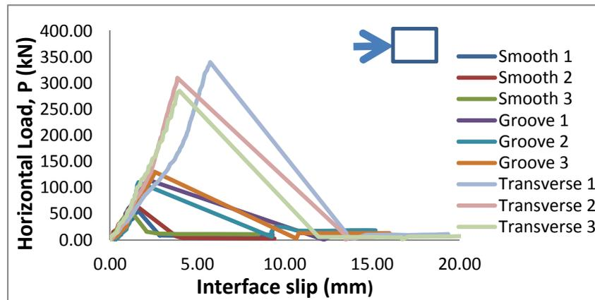
Figure 4. Horizontal load-interface slip relationship for  $\sigma_n = 0\text{ N/mm}^2$
