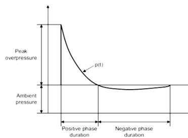
Figure 1. A schematic of the blast wave
