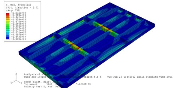
Figure 10: Results of HAT stiffener thickness of 8.5 mm
