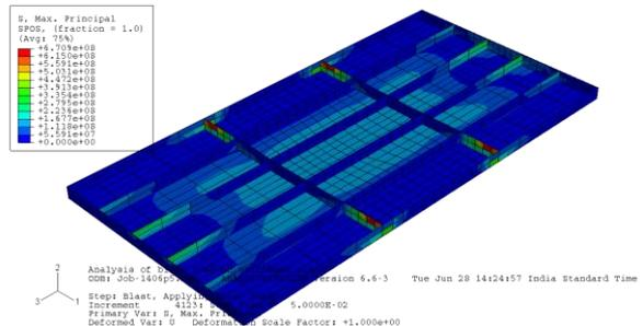
Figure 4: Results of T stiffener thickness of 6.5 mm
