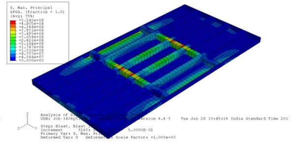
Figure 8: Results of HAT stiffener thickness of 6.5 mm
