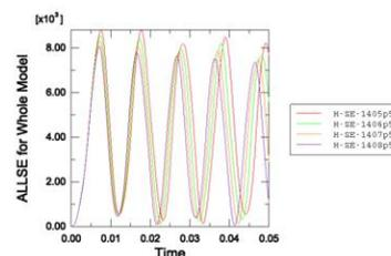
Graph 7: Energy (kNm) vs Time (s) for HAT stiffener with varying thickness
