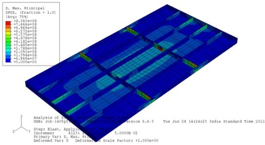
Figure 3: Results of T stiffener thickness of 5.5 mm
