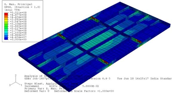
Figure 5: Results of T stiffener thickness of 7.5 mm
