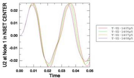
Graph 4: Deflection (m) vs Time (s) for T stiffener with varying thickness
