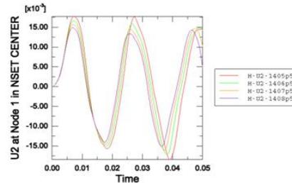
Graph 5: Deflection (m) vs Time (s) for HAT stiffener with varying thickness
