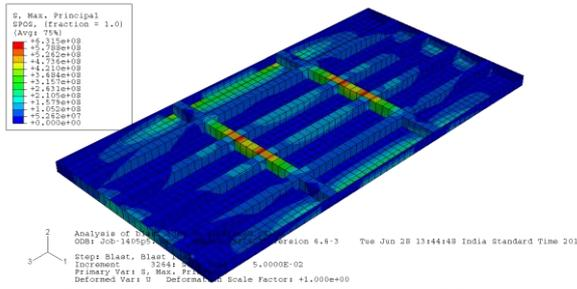
Figure 7: Results of HAT stiffener thickness of 5.5 mm
