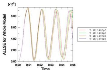
Graph 6: Energy (kNm) vs Time (s) for T stiffener with varying thickness
