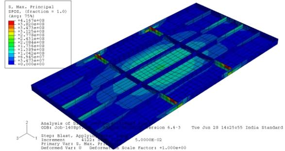
Figure 6: Results of T stiffener thickness of 8.5 mm
