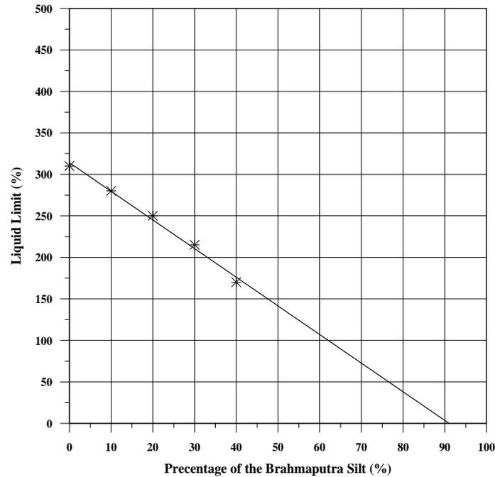
Figure 2. Influence of addition of the Brahmaputra on the Liquid Limit of Bentonite-Silt mixture
