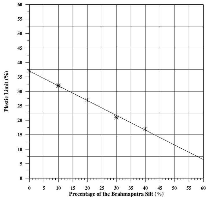
Figure 3: Influence of addition of the Brahmaputra on the Plastic Limit of Bentonite-Silt mixture
