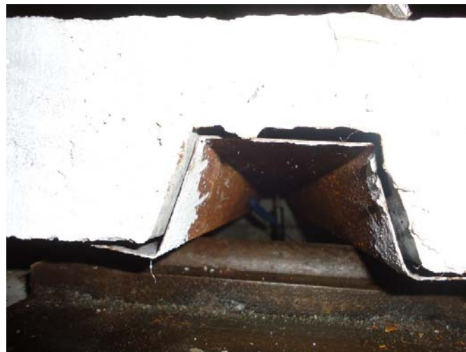
Figure 7. Slip of Trapezoidal Profile sheet slab
