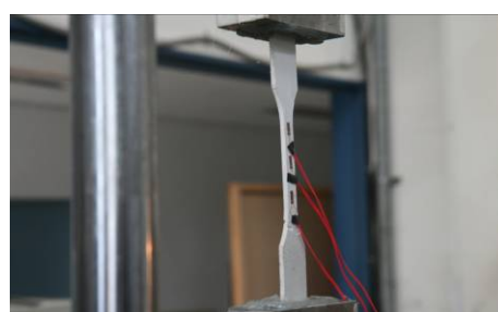
Figure 20 Partial failure on transitional section
