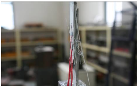
Figure 19 SLE-1 & SLE-2 : Typical tensile failure
