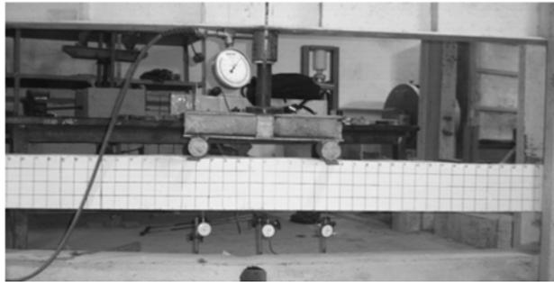
Figure 4 Setup of beam specimen
