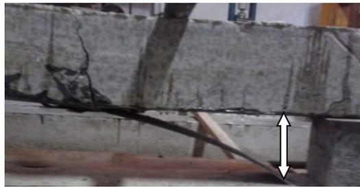
Figure 1 Debonding failure of GFRP sheet on a concrete beam
