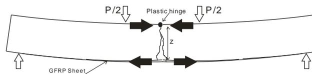
Figure 9 Illustration of the couple moment action after concrete crushing
