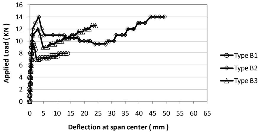
Figure 6 Load-deflection relationship up to final debonding
