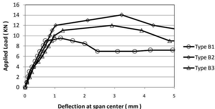
Figure 5 Load-deflection relationship up to Maximum load
