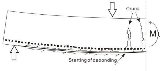
Figure 7 Interfacial debonding started on a major flexural crack
