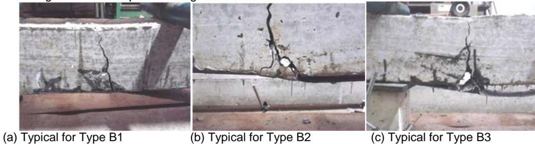
Figure 8 Typical major cracks of specimens
