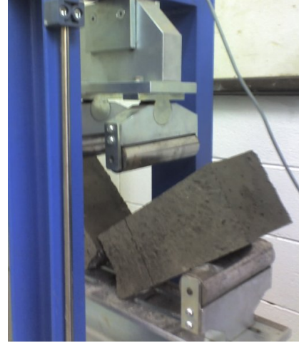
Figure 7. The process of flexural Strength Test
