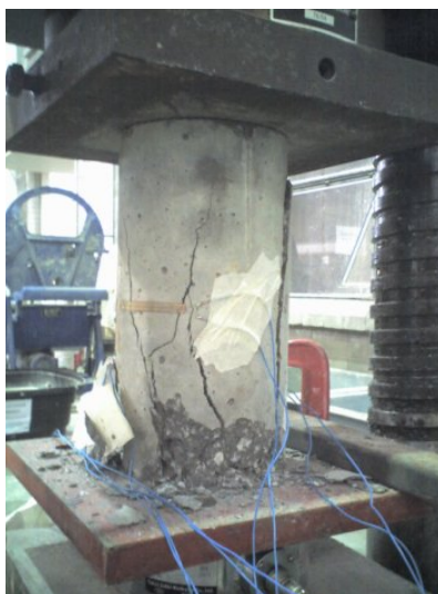
Figure 11. Static modulus of elasticity test
