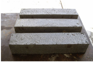
Figure 6. Hardened prism for flexural testing after curing for 28 days
