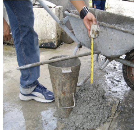
Figure 1. The process of Slump test measurement
