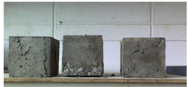
Figure 5. Failure cube after compressive testing in structure lab
