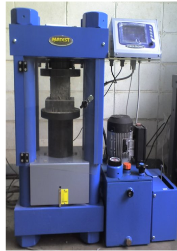
Figure 4. The process of Compressive strength test
