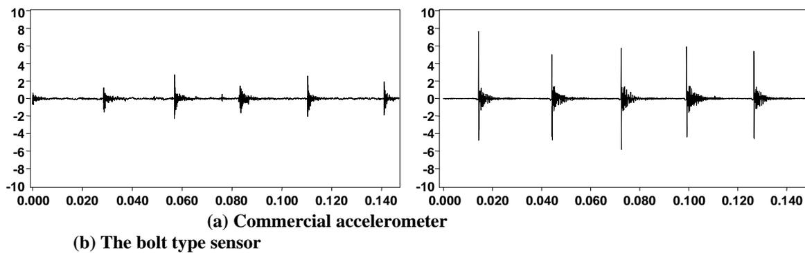
**Fig 4. Defective bearing signals**
