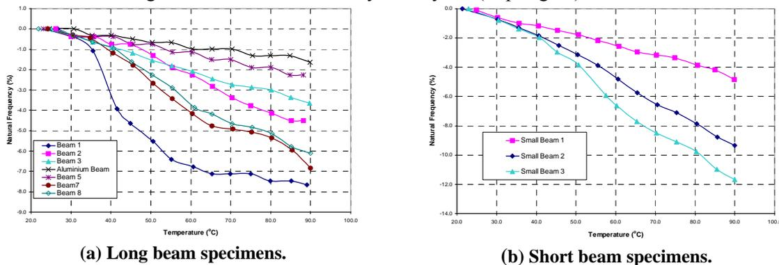
Fig 2. Percentage deviation in first natural frequency of beam specimens with temperature (Ref 26°C).
