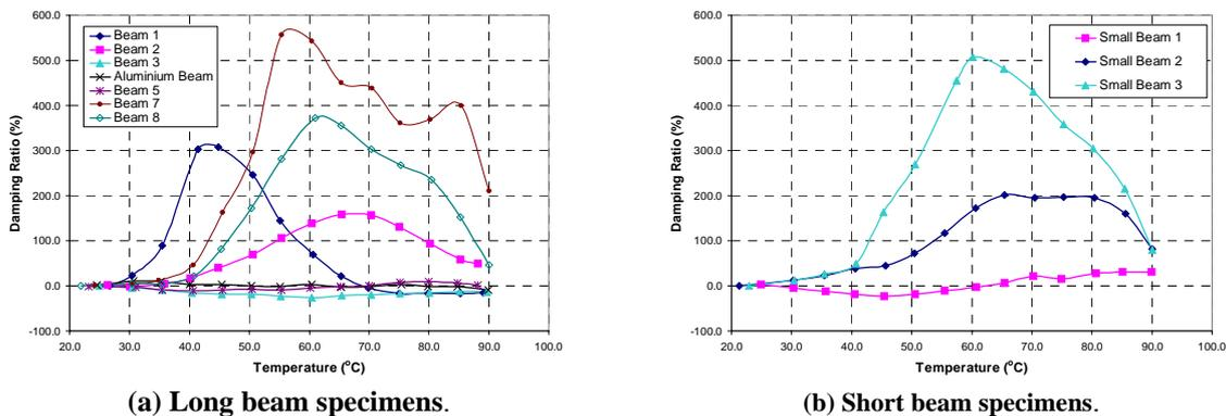
Fig 3. Percentage deviation in free-vibration damping ratio with temperature (Reference 26°C).
