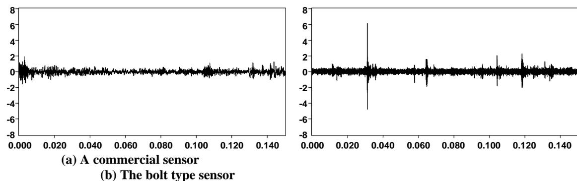
**Fig 5. Damaged bearing signals via a commercial and the bolt type sensor.**
