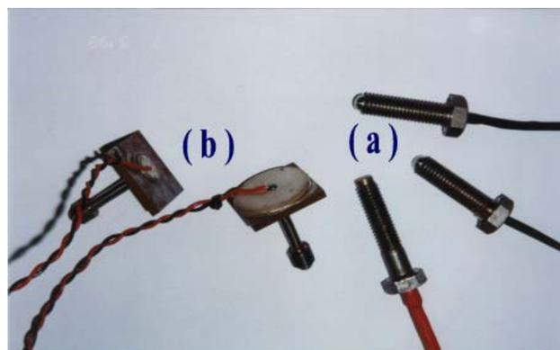
**Fig 1. An enlarged view of the sensors used for vibration detection, (a) Bolt type and (b) Probe type.**
